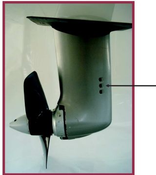
1.1. S-drive engine sea water inlets..
