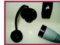
Windlass controller socket
