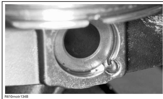
CORRECT POSITION OF THE PISTON CIRCLIP
