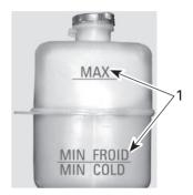
Level between marks when engine is B00067 cold
