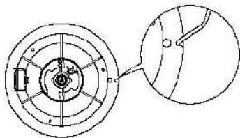
2. Pull the starter rope completely.
