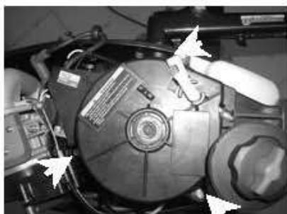
4. Assemble two bolts to fix the fuel tank.
