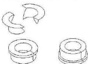
9. Inspect: whether the tilt lock bracket and tilt locked clasp were distorted, replace if needed.
