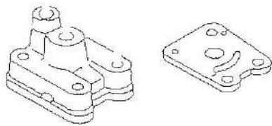
6. Check inner water pump cover and impeller for crack, deform, burn or damage. Replace if necessary.
