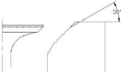
4. If the valve seal surface is too narrow and on the bottom edge of valve surface, use 60° cutter to adjust the bottom edge of the seat, and use 45° cutter to adjust the valve seat width if necessary.
