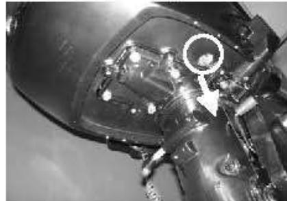
2. Install new gasket and washer, install drain plug.
