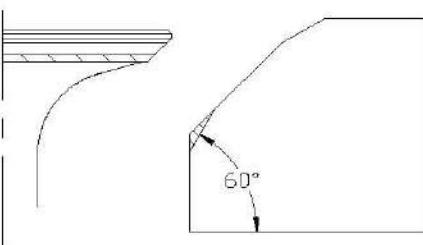
5. Coat evenly a thin layer of lapping compound onto valve seat, and lap the valve by lapping tool.
