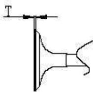
3. Inspect the valve stem diameter. If not in the prescribed range, replace the valve.
