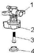
1. Oil switch 2. Thumb wheel 3. Plus pan head screw M4X12 4. Thumb wheel block
