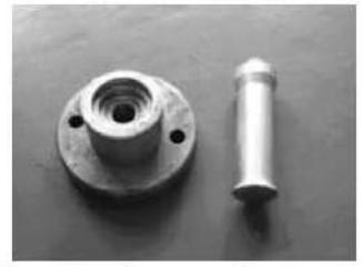
Lower casing cover bearing installer
