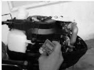
3. Turn the throttle stop screw clockwise or counter clockwise, until the specified idling speed is attained.
