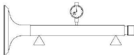
5. Measure the inner diameter of the valve pipe.
