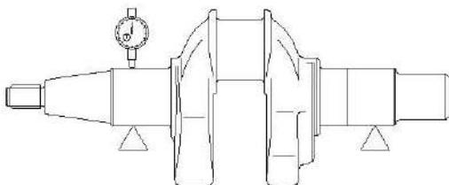
Crankshaft runout limit: 0.03mm
