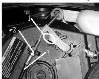
1. Triangle marking 2. Adjusting nut 3. Tightwire ass'y, detent
