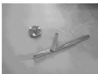
2. Check if the flywheel is damaged or the permanent magnet part is firm. Replace if necessary.
