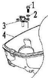
1. Screw 2. Gasket 3. Oil switch 4. Bottom cowling
