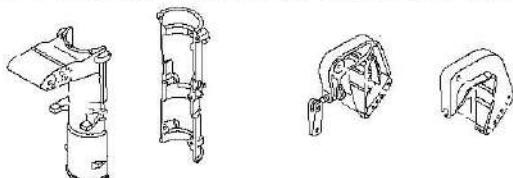
8. Inspect the bush and shock absorption for damage or crack. Replace if necessary.
