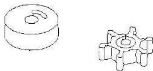
7. Check water pump base for crack, crank, scratch or damage. Replace if necessary.
