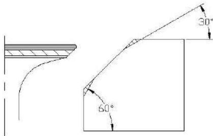
3. If the valve seat is too narrow and on the top edge of valve surface, use 30° cutter to adjust the top margin of the seat, and use 45° cutter to adjust the valve seat width if necessary.
