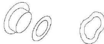
11. Inspect if steering handle shock damper is cracked or damaged. Replace if necessary.
