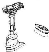
5. Check gear shift handle and change shaft for crack or wear. Peplace if necessary.
