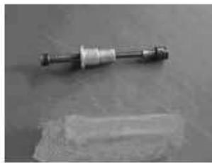
Barrel bearing with guard board installer tool
