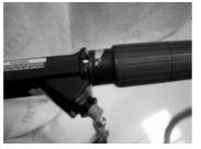
5. Pull out the choke knob fully.
