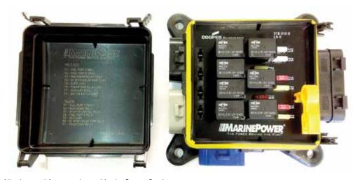
All relays and fuses are located in the Severe Service Vessel Electrical Center (SSVEC). This enclosure is capable of withstanding direct water spray. Additionally, it contains a Goretex vent which allows humid vapors to escape without allowing water in.
