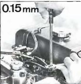
Valve-rocker arm clearance setting: Remove rocker arm cover - With cold engine set both valve tappet clearance to 0.20 mm. after turning flywheel until piston reaches T.D.C. on compression stroke - Tighten adjusting screw locking nuts.
