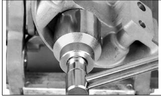
Fill the swivel bracket wit h Triple-Guard grease through the gre ase fit ting on the bracket's port side. Lubricate the tilt tube, swivel bracket, and stern brackets through the two forward grease fittings.
