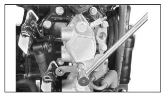
**Tighten Screws in Stages**
