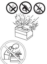
Never remove charger cables from battery posts. It is a sure way to make a lot of sparks in an area surrounded by battery gas.
