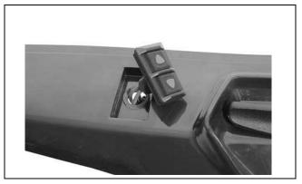
Install nut on switch. Tighten nut to a torque of 10 to 16 in. lbs. (1 to 2 N·m).
