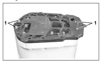
1. Adapter retaining screws
