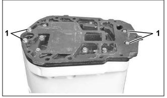
1. Adapter retaining screws
