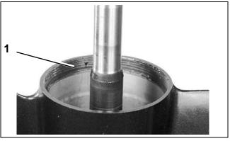
1. Hydrostatic seal grooves
