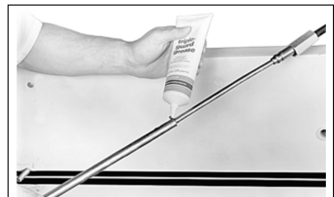
ABYC-approved mechanical steering cable.
