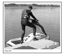
**NOTE:** When boarding a watercraft with the "moto" or kart seat configuration, you can use the seat as an additional support point to keep your balance.
