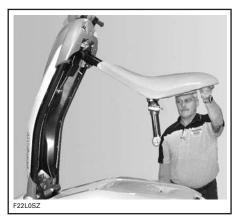
Rotate the post to a vertical position and move the seat to line up the post with its receiver.
