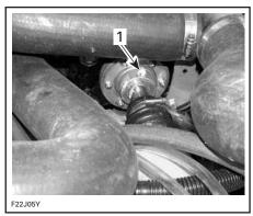
1. Grease seal carrier of mid bearing
