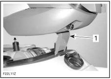
1. Steering pole retainer locked
