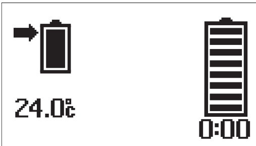
Full charging for operation of the craft complete
