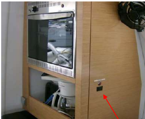
Press this button to open the solenoid
