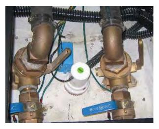
The photo shows the Crash Valve are closed (handle is perpendicular to the flow), and the Seawater intake valves are open (UP position is OPEN). This is the normal operating position of these valves. In this position the seawater comes through the Seawater Intake Valve into the Engines and out of the boats exhaust.
