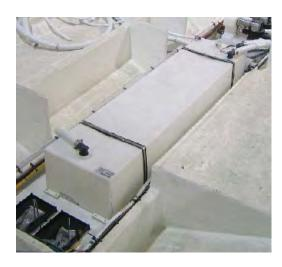
until pumped out at a proper facility. The photo below shows the waste tank. The Waste Tank is equipped with an electronic Waste Level Gauge, which monitors the volume of waste in the tank for your convenience in determining when pumpout is required. The photo below shows the Meter in the Salon.
