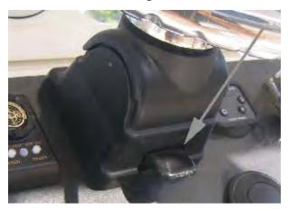
On the Top is the vented fill cap. The photo below shows the vented cap.
