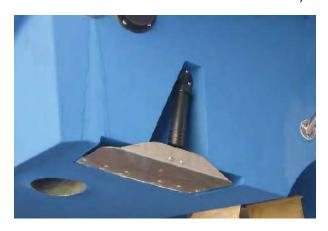
Each Trim Tab operates independently of each other and they are controlled by separate rocker-type switches, located on the Helm Switch Panel (Refer to the Electrical Pages in this section of this Owner's Manual for the location of these switches). Each Trim Tab is actuated by a hydraulic cylinder, which moves them in an Up or Down motion.
