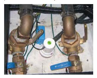
The photo above shows two sets of valves. The upper set of valves, closest to the bilge pump, are the seawater intake valves. The lower set of valves are the crash valves. It is very important to know the various combinations of these valve settings. The wrong combination of setting could sink your vessel. The photo above shows the normal operating positions. The Seawater Valves are open and the Crash valves are closed.
