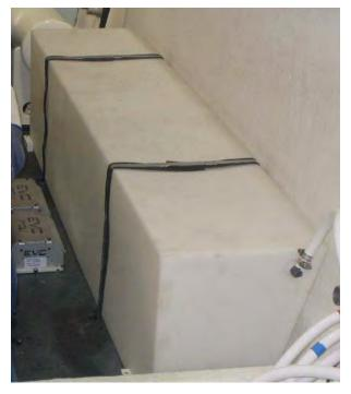
The fresh water tanks are located in the engine room. There are two tanks, one on the outboard side of each engine. The Mechanical Schematic in the SCHEMATICS SECTION of this manual shows the location of the fresh water tanks. They are filled through a fill fitting that is marked "WATER" on the fill cap, which is located on the port side of the deck. The photo below shows the water fill.
