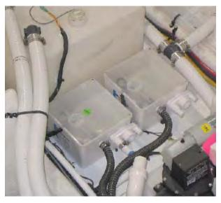
Access to the Shower Sump Pump is through a hatch located on the passageway floor. The photo below shows the panel removed.
