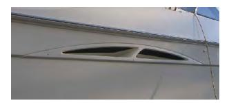
This is an always open vent that has no fan attached to it.
