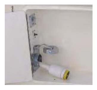
Main Panel, it goes through a Breaker in the cockpit. This Breaker is located inside the same compartment as the Shore Power Hook-Up. The Power then goes to the ISO Transformer. The isolation transformer will electrically isolate the AC Shore Power from your boats AC power system. This eliminates any worries of hooking the boat up to unknown sources of shore power. From the ISO Transformer, the 240 Volt Power goes to the Shore Power/Generator Slide Switch at the AC Main Panel in the Salon.
