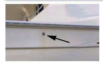
The fuel tank is vented. The photo above shows the fuel tank vent on the starboard side.
