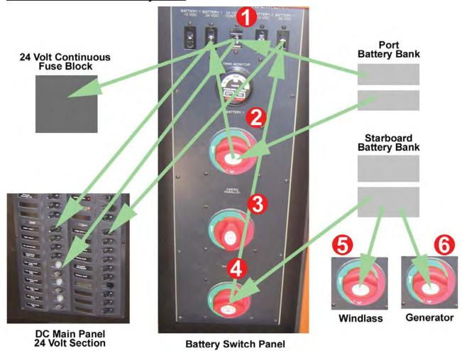
The photo above shows the main components of the 24 Volt Electrical Power System on your **45C**. It is important you understand what the 6 switches above do.
