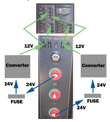
All 12 Volt Power to your vessel is converted from 24 Volt Power. This conversion takes place in three separate instances on your vessel. The drawing above displays the 24 volt to 12 volt power conversion in two of the three instances and where it flows.
