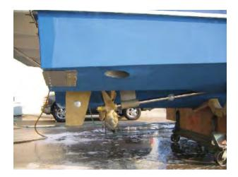
A large sacrificial zinc anode plate is also attached to the underwater area of the transom.
