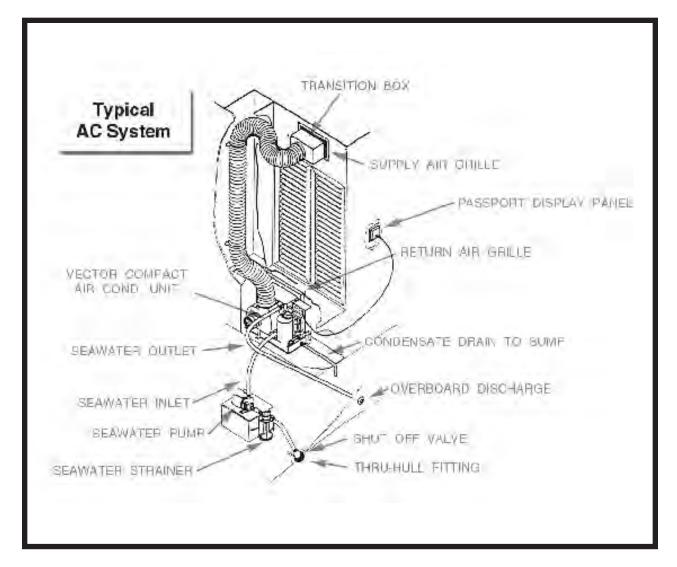
Each air conditioning unit is controlled by an independent thermostatic control panel ("Elite Control"), which is located within the respective cooling/heating zones. The desired zone temperature is manually set on the "Elite Control" and the air conditioning unit is activated to supply cooling or heating as required to constantly maintain the temperature selected. The photo below shows the control.
