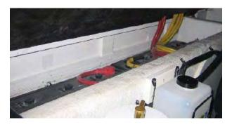
Starboard and Port Battery Banks: Access to the Starboard and Port Battery Banks are under the platform in the engine room, forward of the engines.
