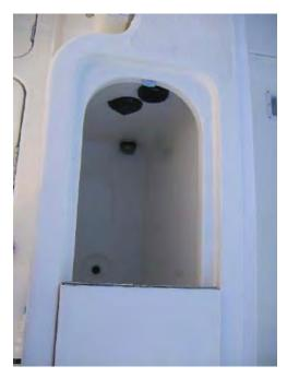
The Live Well system will keep your fish and bait alive. The Live Well system circulates and inserts air into the tank the fish are in.
