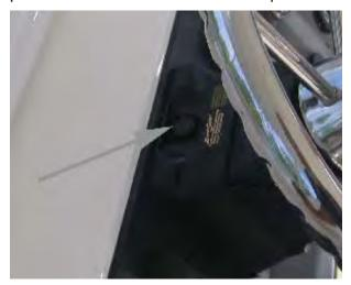
Maintenance of the **Hydraulic Steering System** should only be performed by your Silverton dealer or a qualified technician, who is experienced in marine hydraulic systems. Periodically examine all connections and hydraulic lines for any signs of leakage. If any leaks are noted, contact your Silverton dealer for further inspection and repair, if necessary.
