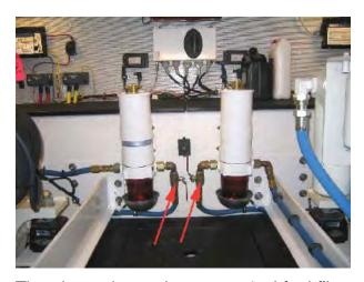
The photo above shows a typical fuel filter system for the diesel engines. Arrows on the photo indicate Fuel Shut-Off Valves. Each engine has a separate fuel filter and fuel shut-off valve located near the engine. The fuel filter is located forward of the engines.
