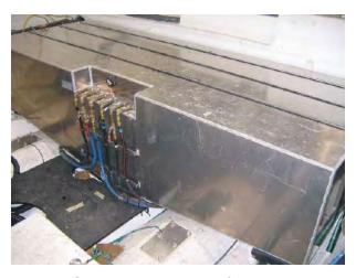
Your **45C** is equipped with a fuel tank having a capacity of 607 gallons. See the Mechanical Schematic in the SCHEMATICS Section of this Owner's Manual for the location of the fuel tank.
