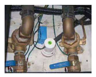
The photo above shows an unacceptable combination of valve settings. The Seawater Intake Valves are closed, and the Crash Valves are closed. The engine CAN NOT run in this condition. There is NO water cooling the engine.
