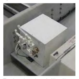
The photo above shows the Water Heater. The Water Heater is accessible from the access panel in the Galley Floor. Operation of the water heater is as follows:
