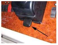
The steering head contains a vented fill cap. The vented cap is located on the top of the steering head and forward of the steering wheel. The photo below shows the vented cap.
