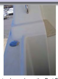
The photo above shows the Port Fuel Tank Fitting. It is located on the gunwale in the cockpit. The Starboard Fuel Tank Fitting is located in the same position, but on the starboard side. The fuel fill fittings are connected to the fuel tanks with the fuel hoses.
