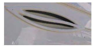
This is an always open vent that has no fan attached to it.
