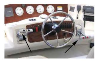
The transmissions are counter-rotating. This is defined as when in the forward shift mode and viewing forward from aft, the Port transmission rotates the Port propeller counterclockwise and the Starboard transmission rotates the Starboard propeller clockwise.
