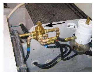
If your **38SB** is diesel powered, the generator fuel selector Valve also determines the tank to which the unused fuel is returned. This fuel is always returned to the same tank that is supplying the fuel to the generator.
