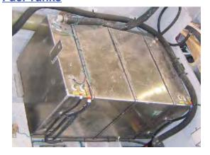
Your **38SB** is equipped with two (2) fuel tanks, each having a capacity of 186 gallons, for a total fuel capacity of 372
