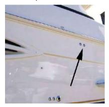
The starboard vent is in the same location on the other side of the hull. The vent fittings are connected to the fuel tanks with the fuel vent hoses. These vents allow air to pass through them when fueling and when the engines are drawing fuel from the tanks.
