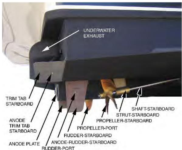
The **Shaft** is connected to the engine transmission with a coupling and extends through the bottom of the hull. The **Propeller** is attached to the end of the shaft. The shaft is supported forward of the propeller by **Strut**. The struts support and stabilize the shafts. The rotation of the
