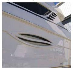
For quicker evacuation of air from the engine room, your **38SB** is equipped with two (2) bilge blowers. The blowers are located in the engine compartment and exhaust out through the deck on the port and starboard sides of your **38SB**. The photo below shows the blower exhaust on the starboard side of your **38SB**.
