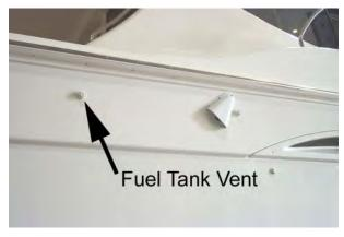
The port side vent is in the same location on the other side of the hull. The vent fittings are connected to the fuel tanks with the fuel vent hoses. These vents allow air to pass through them when fueling and when the engines are drawing fuel from the tanks.
