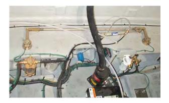
The **Hydraulic Steering System** in your **38C** utilizes fixed-type steering head.
