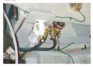
If your **38C** is diesel powered, the generator fuel selector Valve also determines the tank to which the unused fuel is returned. This fuel is always returned to the same tank that is supplying the fuel to the generator.
