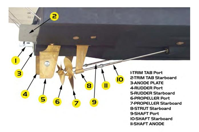
The **Shaft** is connected to the engine transmission with a coupling and extends through the bottom of the hull. The **Propeller** is attached to the end of the shaft. The shaft is supported forward of the propeller by two **Struts**. The struts support and stabilize the shafts.
