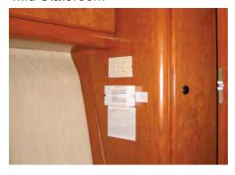
Each CO monitor is operated by DC electrical power and they are connected directly to the batteries. It is not necessary for the battery switch to be turned ON for them to operate. The fuses for the monitors are located behind the AC/DC Panel.
