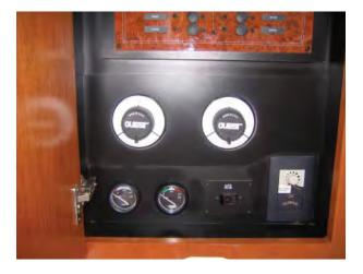
The positions on the battery switch are ON and OFF. The switch must be turned to the ON position to supply power to the DC electrical system. When the battery switch is turned to the OFF position, power is disconnected to the DC electrical system.
