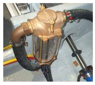
If your **38C** is equipped with a generator, a remote fuel filter with a fuel shut-off valve is located in the main generator fuel supply line, separate from the engine fuel supply lines. The photo below shows the generator fuel filter.
