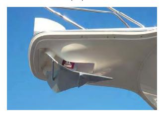
The photograph below displays the optional Anchor Windlass and controls, which are located on the forward section of the deck immediately aft of the pulpit.
