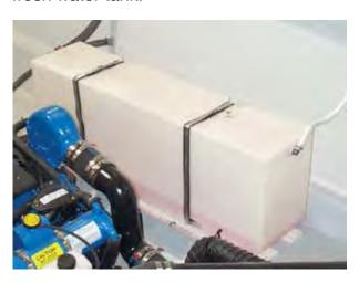
The Mechanical Schematic in the SCHE-MATICS SECTION of this manual shows the location of the fresh water tanks. They are filled through a fill fitting that is marked "WATER" on the fill cap, which is located
