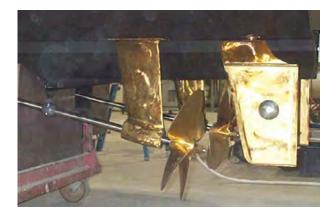
A large sacrificial zinc anode plate is also attached to the underwater area of the transom.
