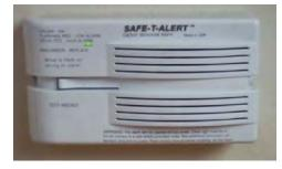
Operation of the CO monitors requires a ten (10) minute warm-up period, during which time, the sensor element is cleaned and the unit is stabilized. During this ten minute warm-up period, the GREEN indicator light will flash ON and OFF. The GREEN indicator light will remain ON after the completion of the warm-up period until the presence of Carbon Monoxide Gas
