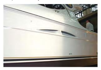
For quicker evacuation of air from the engine room, your **38C** is equipped with two (2) bilge blowers. The blowers are located in the engine compartment and exhaust out through the hull on the port and starboard sides of your **38C**. The photo below shows the blower exhaust on the starboard side of your **38C**.
