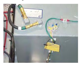
The Fuel Tanks should be inspected for signs of leaks, corrosion, and/or pitting at least once a year. Corrosion normally appears as a white chalky, discolored or flaky appearance on the surface of the tank. Sometimes it also appears as pitting or small pockets of missing aluminum. Another indication of corrosion could be bubbles on the paint that coats the fuel tank. If any one of theses conditions are
