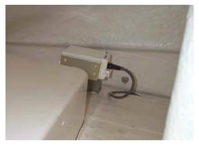
The SatCom Sending Unit is installed under the flybridge on your yacht. This unit sends out a low frequency signal to the satellite, which in turn sends the signal to the receiving location. You must know the location of the Sending Unit. If anyone is standing in front of the Sending Unit, they could block the signal from going to the satellite. Refer to the SeaKey Owners Guide for more information.
