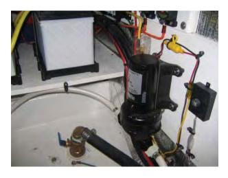
Fresh Water Lines (Cold Water and Hot Water): The fresh water lines carry the water from the fresh water tanks, the water heater, and the various faucets located in the Galley and Head areas of your 38C. They are constructed of polybutylene plastic material and are 1/2 inch inside diameter. The COLD WATER lines have pale blue manufacturer's lettering and the HOT WATER lines have pale red
