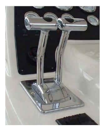
The transmissions are counter-rotating. This is defined as when in the forward shift mode and viewing forward from aft, the Port transmission rotates the Port propeller counterclockwise and the Starboard transmission rotates the Starboard propeller clockwise.
