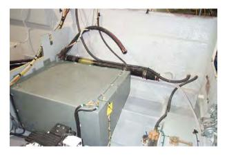
Your **38C** is equipped with two (2) fuel tanks, each having a capacity of 188 gallons, for a total fuel capacity of 376
