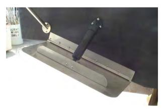
Each trim tab operates independently of each other and they are controlled by separate rocker-type switches, located on the Helm Switch Panel (Refer to the Electrical Pages in this section of this Owner's Manual for the location of these switches). Each trim tab is actuated by a hydraulic cylinder, which moves them in an Up or Down motion.
