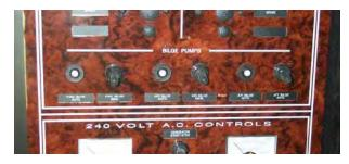
BREAKER SWITCHES: The breaker switches are your safety switches. They work just like a fuse, but are resetable. If the breaker switch is activated, before resetting the switch, locate the problem. The breaker is reset by pushing in the white button.
