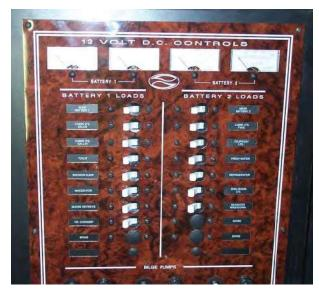
There are four meters across the top of the panel. These meters show the yachts battery condition. They are (from left to right):
