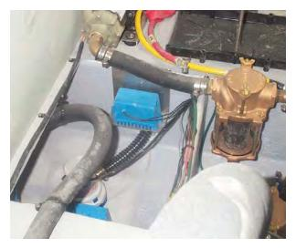
Access to the High Water High Water Switch is through the panel in the Galley Floor. Please be aware this Alarm Switch is about 5" higher than the normal operating bilge switches that are installed on your yacht by Silverton. Please also be advised that the switch is only in the mid compartment. Other compartments could flood first and the switch would not be activated. The switch will only be activated when the normal operating bilge pumps
