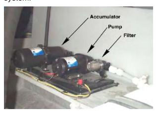
Fresh Water Lines (Cold Water and Hot Water): The fresh water lines carry the water from the fresh water tank, the water heater, and the various faucets located in the Galley and Head areas of your 35MY. They are constructed of polybutylene plastic material and are 1/2 inch inside diameter. The COLD WATER lines have pale blue manufacturer's lettering and the HOT WATER lines have pale red manufacturer's lettering for identification purposes. The fresh water lines require
