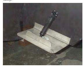
Each trim tab operates independently of each other and they are controlled by separate rocker-type switches, located on the Helm Switch Panel (Refer to the Electrical Pages in this section of this Owners manual for the location of these switches). Each trim tab is actuated by a hydraulic cylinder, which moves them in an Up or Down motion.
