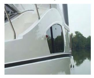
The Port Navigation Light is RED. The Starboard Navigation Light is in the same position but on the starboard side of the boat. The Starboard Navigation Light is green.
