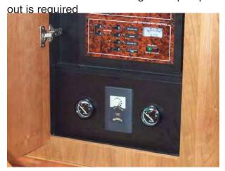
Maintenance of your *Sea Land* Vacu-Flush Sanitation System consists of periodic cleaning of the toilet bowl with a mild nonabrasive cleaner. The Waste Tank should be thoroughly rinsed after each pump-out and a sanitation system deodorizer should be added to the Waste Tank by flushing through the toilet.
