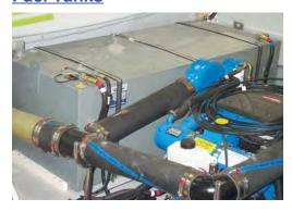
Your **35MY** is equipped with two (2) fuel tanks, each having a capacity of 143 gallons, for a total fuel capacity of 286 gallons. The photo above shows the port side
