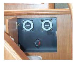
The positions on the battery switch are ON and OFF. The switch must be turned to the ON position to supply power to the DC electrical system. When the battery switch is turned to the OFF position, power is disconnected to the DC electrical system.
