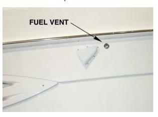
The starboard side vent is in the same location on the other side of the hull. The vent fittings are connected to the fuel tanks with the fuel vent hoses. These vents allow air to pass through them when fueling and when the engines are drawing fuel from the tanks.
