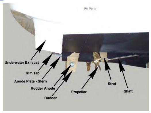
The **Shaft** is connected to the engine transmission with a coupling and extends through the bottom of the hull. The **Propeller** is attached to the end of the shaft. The shaft is supported forward of the propeller by a **Strut**. The struts support and stabilize the shafts.
