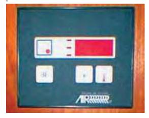
Each air conditioning unit will operate in a "**Dehumidification**" mode upon demand and is controlled by the "Passport Control". Refer to the *Marine Air Systems* Operation and Maintenance Manual for a complete description and instruction in the operation of this mode.
