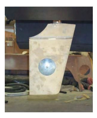
A large sacrificial zinc anode plate is also attached to the underwater area of the transom.
