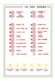
The left hand side are all the switches connected to battery #1. The right hand side are all the switches connected to Battery #2.
