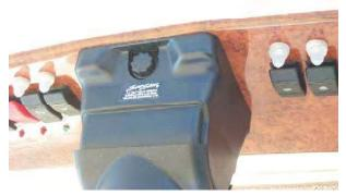
Maintenance of the **Hydraulic Steering System** should only be performed by your Silverton dealer or a qualified technician, who is experienced in marine hydraulic systems. Periodically examine all connections and hydraulic lines for any signs of leakage. If any leaks are noted, contact your Silverton dealer for further inspection and repair, if necessary.
