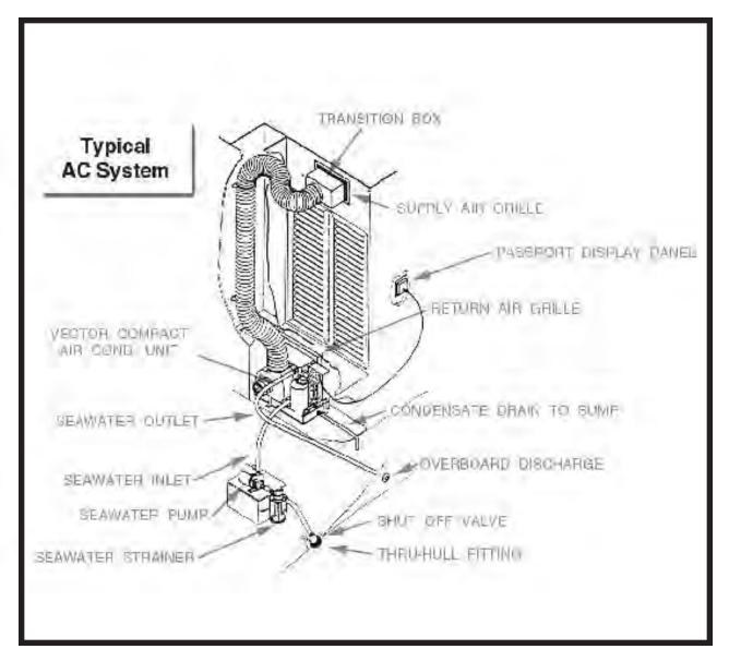
Each air conditioning unit is controlled by an independent thermostatic control panel ("Passport Control"), which is located within the respective cooling/heating zones. The desired zone temperature is manually set on the "Passport Control" and the air conditioning unit is activated to supply cooling or heating as required to constantly maintain the temperature selected. The photo below shows the salon control.
