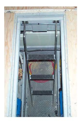
The Engine Compartment is accessed through the Access Panels in the Salon Deck. The photo below shows the panels removed.
