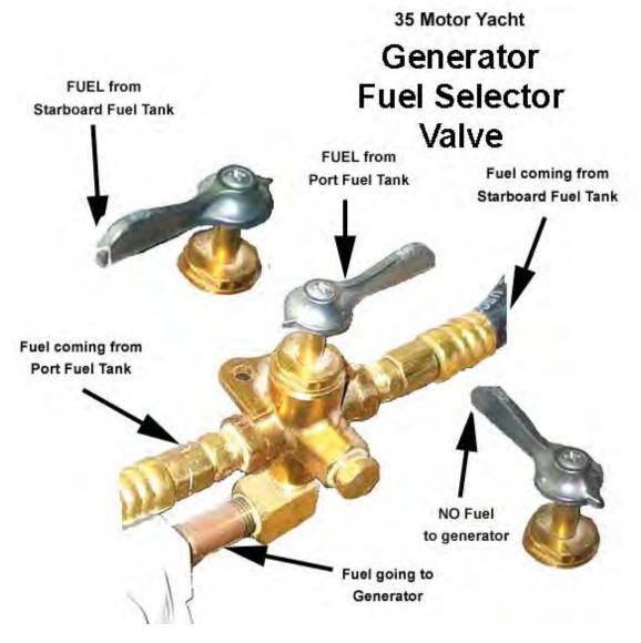
If your **35MY** is equipped with a generator, a fuel tank selector valve is located on the aft bulkhead of the engine compartment. This valve determines the tank from which the generator will draw its fuel from. The photo above shows the Fuel Selector Valve.
