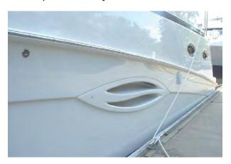
For quicker evacuation of air from the engine room, your **35MY** is equipped with two (2) bilge blowers. The blowers are located in the engine compartment and exhaust out through the hull on the port and starboard sides of your **35MY**. The photo below shows the blower exhaust on the starboard side of your **35MY**.
