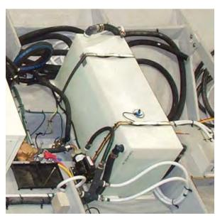
The Waste Tank is equipped with an electronic Waste Level Gauge, which monitors the volume of waste in the tank for your convenience in determining when pump-
