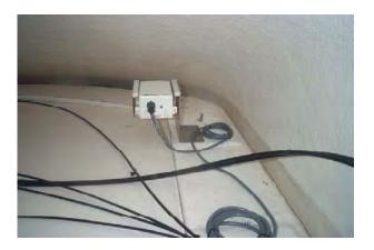
The SatCom Sending Unit is installed under the helm on your yacht. This unit sends out a low frequency signal to the satellite, which in turn sends the signal to the receiving location. You must know the location of the Sending Unit. If anyone is standing in front of the Sending Unit, they could block the signal from going to the satellite. Refer to the SeaKey Owners Guide for more information.
