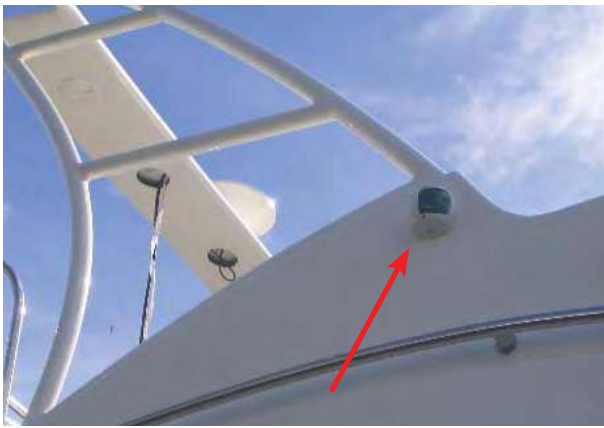
The Starboard Navigation Light is GREEN.
