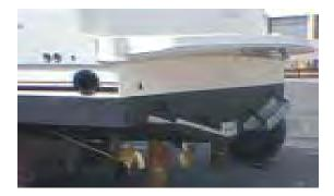
The **Shaft** is connected to the engine transmission with a coupling and extends through the bottom of the hull, where it is connected to the propeller. The shaft is supported forward of the propeller by a **Strut**. The struts support and stabilize the shafts. The rotation of the **Propellers** propel the yacht in the selected direction, controlled from the helm station.
