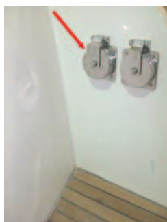
Shore power socket 220V - 32A (Reference 1)
