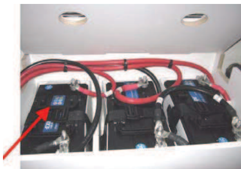
Service batteries: 3 x 80A Spare service batteries: 1 x 80A
