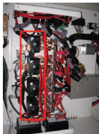
Location - Battery switch: Engine compartment
