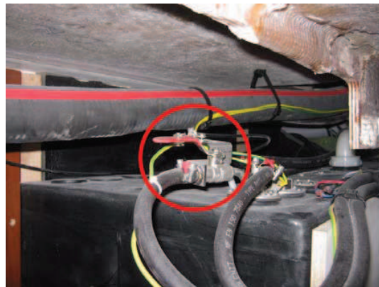
Sea water inlet valve for engine (located directly on sockets)
