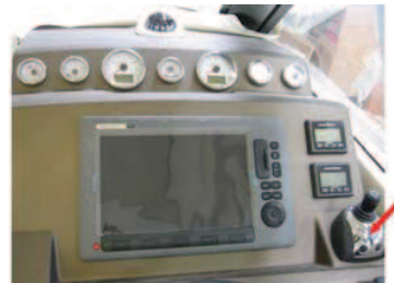
Joystick (For manoeuvring vessel at low speed)
