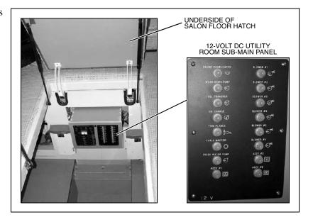
The salon sub-main breaker panel is located inside the electrical cabinet in the port aft corner of the salon.
