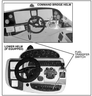
If the pump is running, but you are having problems transferring fuel, see if the fuel transfer hose or fuel tank vent hose is kinked or collapsed. If there are no visible signs of a problem, contact your local dealer.
