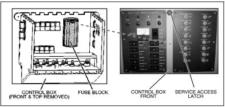
**110-Volt AC Master Panel:** Located inside the electrical cabinet in the port aft corner of the salon.
