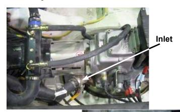
Clean the seawater strainer (located on the left rear of the engine) every 14 days or sooner as conditions warrant.
