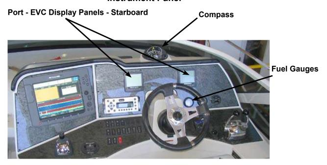
The Volvo Penta EVC system display is an instrument which displays operating information about the engine and allows you to communicate with the engine's electrical system.
