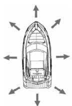
The Joystick controller allows the operator to move the yacht in many more ways than a conventional steering system, including bow thrusters.
