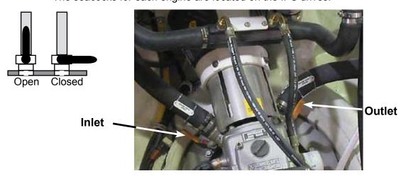
Clean the seawater strainer (located on the left front of the engine) every 14 days or sooner as conditions warrant.
