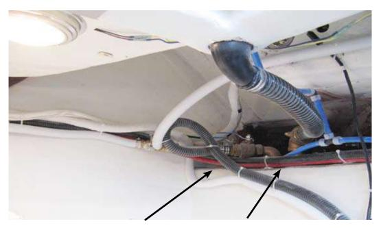
Drains for aft transom area (starboard) shown in open position.
