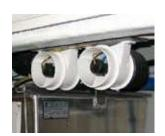
Your boat's engine room is equipped with a ventilation system consisting of intake ducts, exhaust ducts and bilge blowers. This system is designed to remove any fuel vapor and excess heat from the engine room. The bilge blowers operate whenever the engines are running, as long as the four Bilge Blower circuit breakers on the DC Control Panel are ON.
