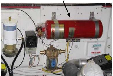
A fire suppression system monitor, installed near the helm, is wired to an ignition switch. The monitor's light should be ON when the ignition switch is turned ON.
