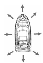
The Joystick controller allows the operator to move the boat in many more ways than a conventional steering system, including bow thrusters.
