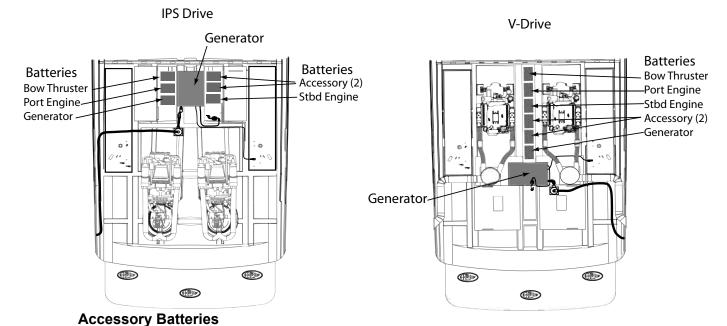
The accessory equipment controlled by the three DC circuit breaker panels (Safety Breaker Panel, DC Control Center and Bridge Breaker Panel) is powered by two batteries. The location of these batteries for the IPS system are on the boat's centerline, forward of the starboard engine battery. For the Inboard system the batteries are located aft of the
