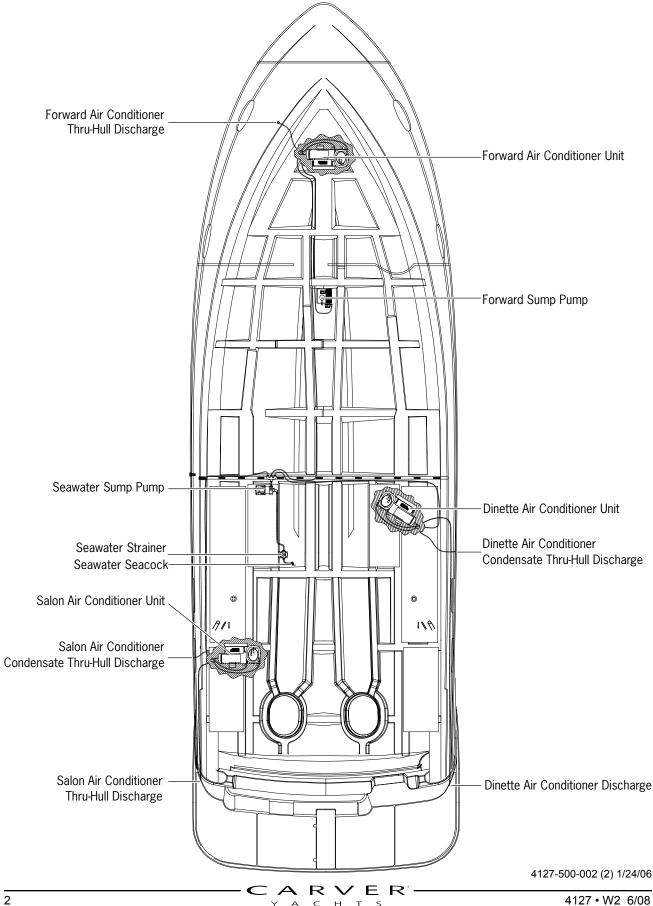
3. Open the air conditioning seacock to supply seawater to the air conditioning pump.
