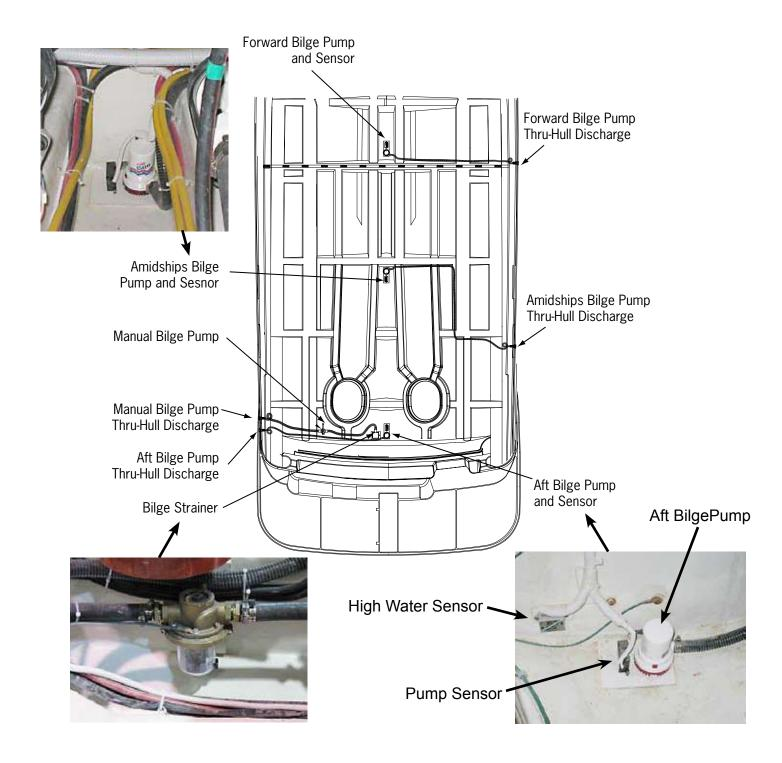
The bilges include the areas described below. Refer to the bilge diagram in this section for the exact location of the bilge pumps.
