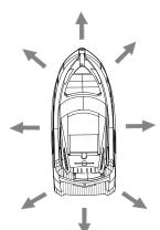
The Joystick controller allows the operator to move the yacht in many more ways than a conventional steering system, including bow thrusters.
