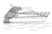
The station wagon effect or back drafting can cause CO gas to accumulate inside the cabin, cockpit or bridge areas when the boat is underway using protective weather coverings. **PRECAUTION:** Provide adequate ventilation when the canvas top, side or back curtains are in their closed, protective positions. Open forward hatch or window.
