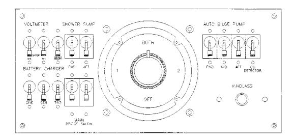
**NOTE:** Since condensation from the air conditioner drains into the shower sump, the shower sump breakers must remain "ON" whenever the air conditioner is operating.
