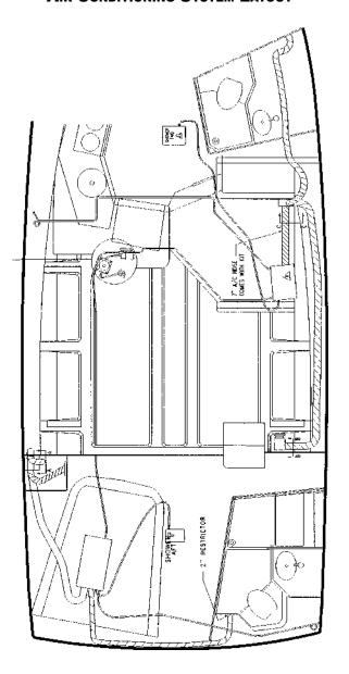
Condensation from this unit drains into the forward shower sump. The second, a 12,000 BTU unit, is installed beneath the aft cabin berth. Condensation from this unit drains into the aft shower sump.
