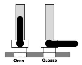
4. Locate the valve that lets you bypass the aft waste tank and flush waste directly overboard. This valve is also located below the aft hatch in the aft stateroom floor. Position the valve to "OVERBOARD".
