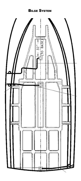
3. The aft bilge starts beneath the aft stateroom floor and runs to the stern. Access the aft bilge pump by lifting the aft-most hatch in the aft stateroom floor. Refer to the "Interior Hatch Locations" portion of Section 9 for more information on bilge pump access.
