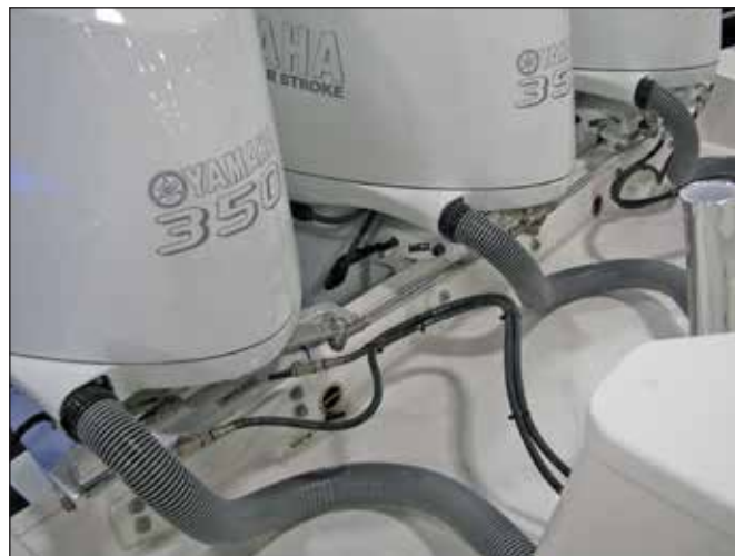
Tie Bars & Dual Steering Cylinders Typical Triple Engine Steering
