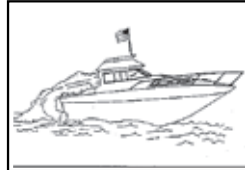
Back Drafting / Station Wagon Effect - at cruising speed with no forward ventilation
