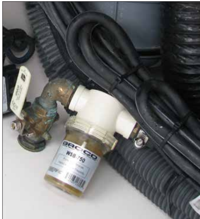
Generator Sea Strainer & Seacock
