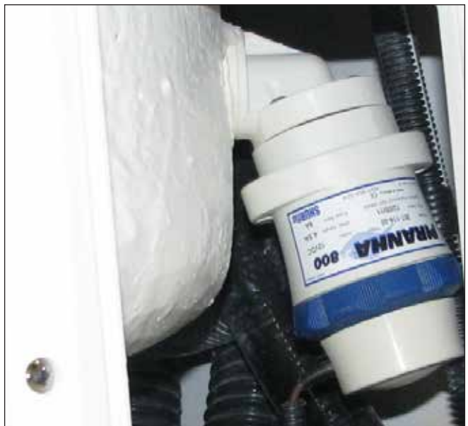
Typical Livewell Recirculation Pump
