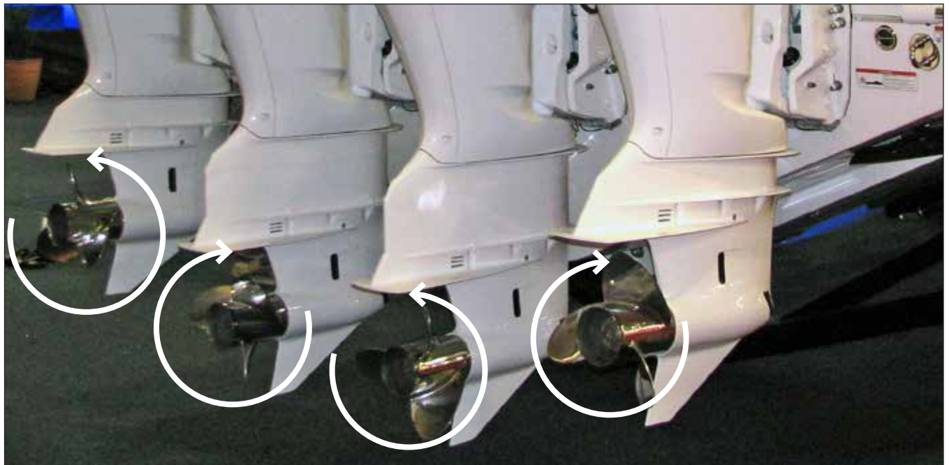
Typical Quad Engine & Propeller Rotation
