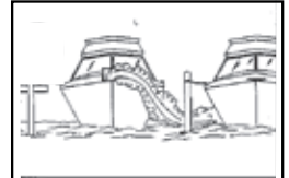
Nearby Generator Exhaust - wind carries exhaust to the other boat
