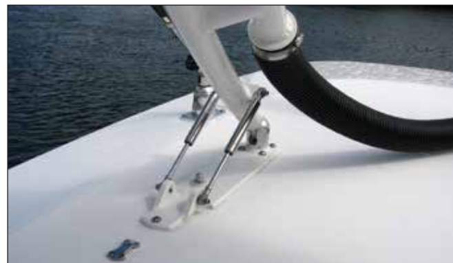
Gas Charged Assist Springs
