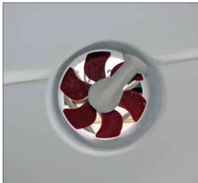
Typical Bow Thruster Drive Unit, propeller & tunnel
