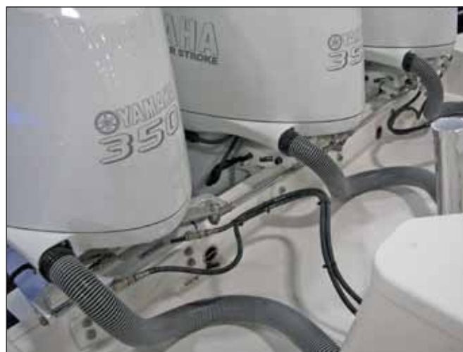
Tie Bars and Dual Steering Cylinders Typical Triple Engine Steering
