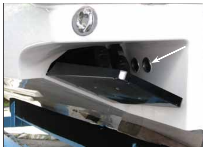
Scupper Drain Thru-hull Fittings
