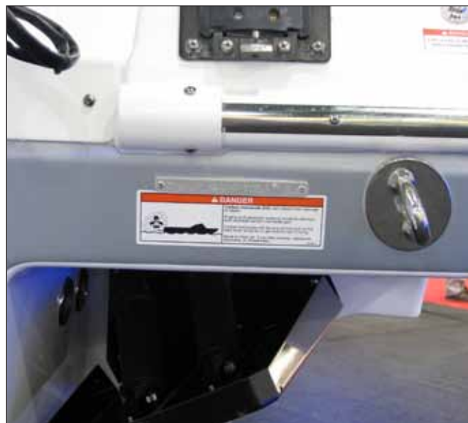
Hull ID # On Starboard Side of Transom
