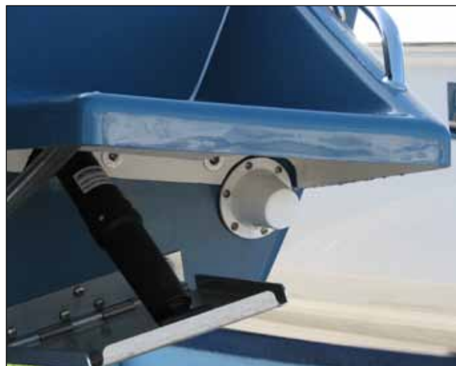
Scupper Drain Check Valve Assembly
