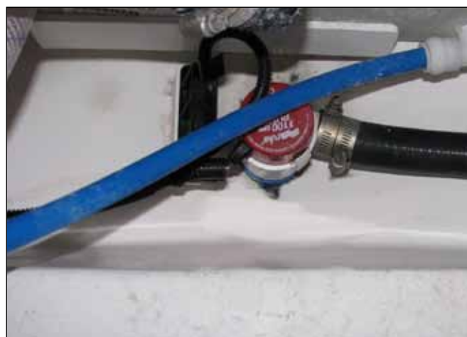
Aft Bilge Pump and Automatic Float Switch
