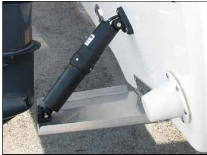
Typical Trim Tab Plane and Actuator
