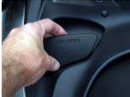
Front compartment with remote release lever
