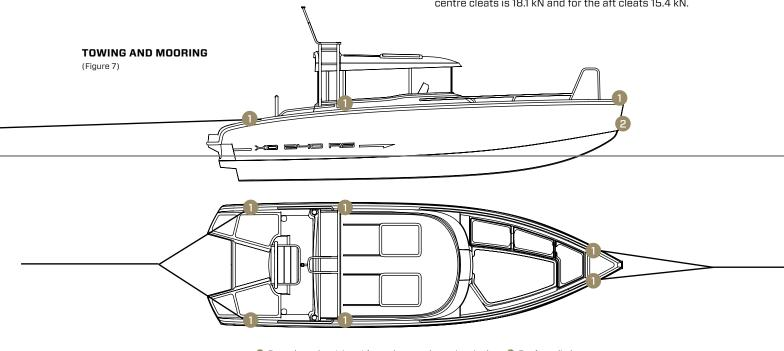
1 Fastening points (cleats) for towing, mooring and anchoring 2 Eye for trailering
