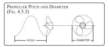
Diameter is that distance measured across the propeller hub line from the outer edge of the 360° that is made by the propeller's blade during a single rotation. Pitch is that distance in inches that a propeller will travel if rotated one revolution without any slippage.
