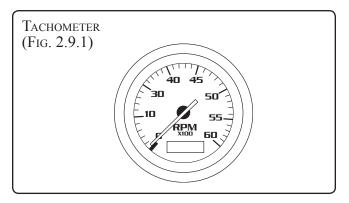
The tachometer indicates the revolutions per minute (RPM) of the engine. (It does not indicate the speed of the boat.) Your Engine Operator's Manual indicates the maximum full throttle RPM at which your engine should operate. This must not be exceeded or serious engine damage will occur. The tachometer should also be used to determine the most comfortable and economical cruising RPM.
