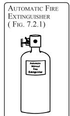
Your boat may be equipped with an automatic fire extinguisher system located in the engine compartment. In the event of a fire, the heat sensitive automatic head will release the extinguishant as a vapor, totally flooding the area in fire-killing concentrations.
