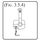
Then move shift/throttle lever rapidly, either forward or reverse, but not very far from the neutral position. The drive unit will engage and boat will start to move slowly in either forward or reverse. You can damage the transmission if you
