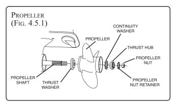
6. Secure the propeller nut by bending three (3) of the tabs of the propeller nut retainer into the thrust hub grooves.
