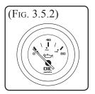
IF OIL PRESSURE GOES ABOVE OR BELOW OPERATING RANGE SHUT DOWN THE ENGINE IMMEDIATELY. GET TRAINED HELP TO FIND AND FIX THE PROBLEM.
