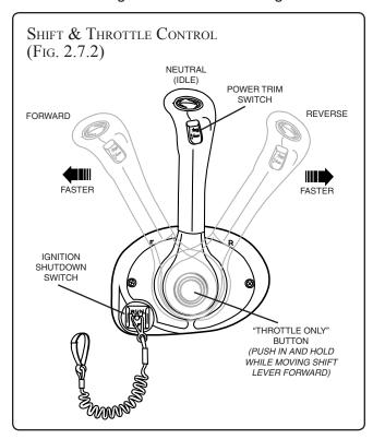
The "throttle only" mechanism may differ from one style gear/throttle unit to another. Refer to your Gear Shift & Throttle Manual for proper operation of this feature.
