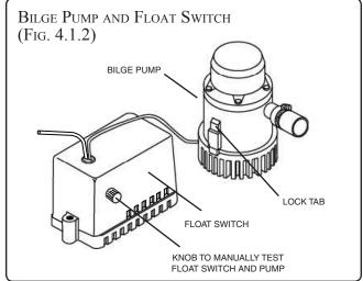
If the liquid level in the bilge is higher than normal and the bilge pump empties the bilge when you use the ON switch, either the breaker for the automatic bilge pump circuit has blown or the float switch is not operating properly. Have it checked immediately. If the ON switch does not operate the pump, DO NOT use the boat until the problem is corrected.
