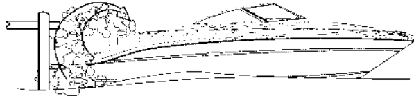
BLOCKING HULL EXHAUSTS. OPERATING AT SLOW SPEED OR DEAD IN THE WATER.
