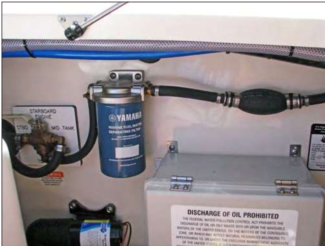
Triple Engine Fuel System - Stbd Engine Fuel Filter, Primer Bulbs & Fuel Selector Valve
