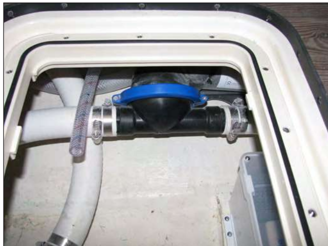
Diaphragm Discharge Pump & Waste Discharge Valve In Forward Cabin Bilge Below Dinette Table
