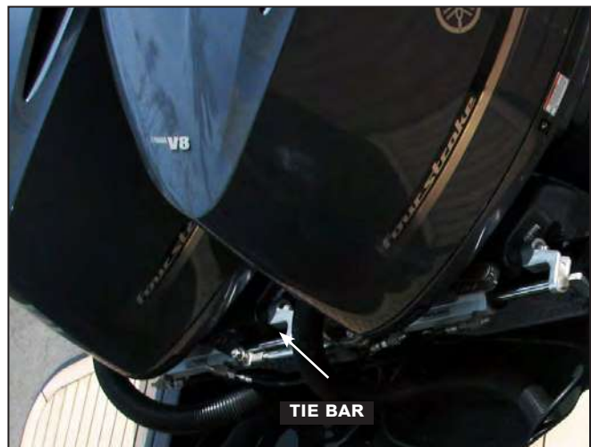
Typical Steering Cylinders & Tie Bar
