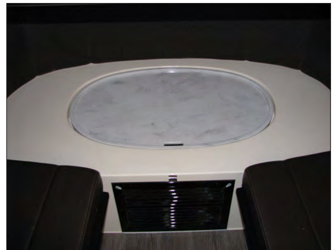
Air Conditioner Compartment Below Forward Dinette Cushion
