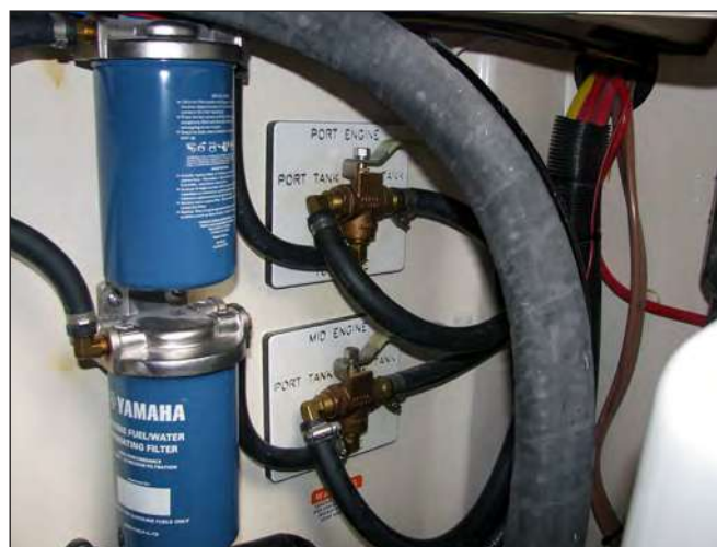
Triple Engine Fuel System - Port & Center Engine Fuel Selector Valves & Filters
