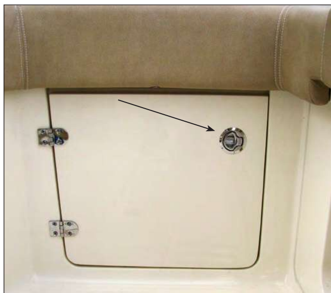
Typical push to close Latch
