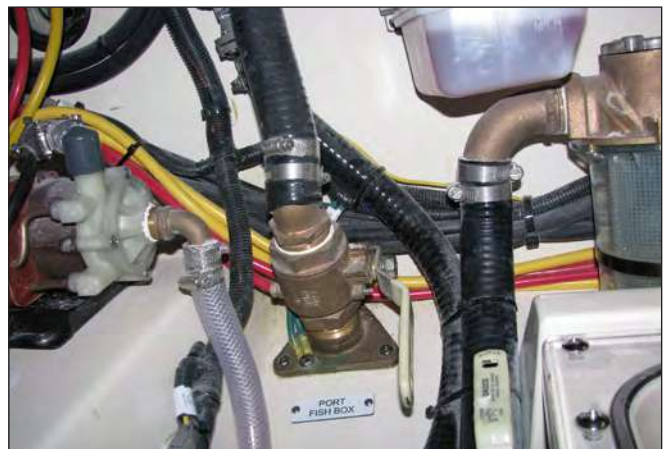
Port Fishbox Pump Out Thru-Hull Fitting & Valve
