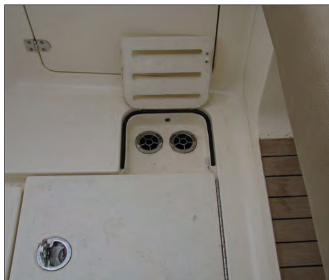
Scupper Drain Thru-Hull Fittings & Check Valves
