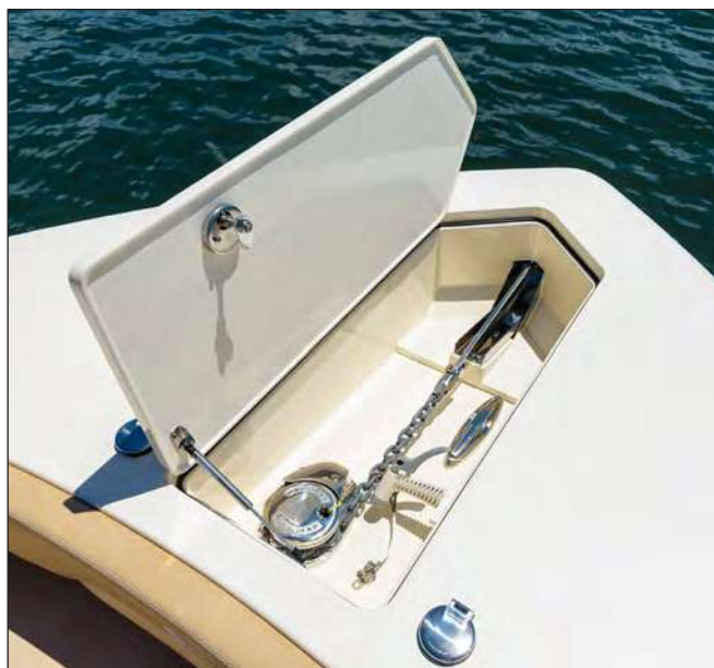
Windlass Compartment Washdown Hose
