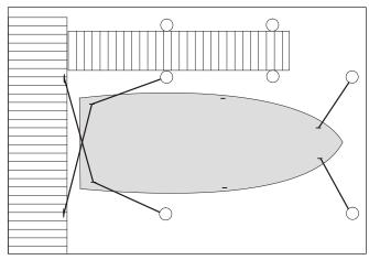
Securing The Boat In A Slip (Typical)
