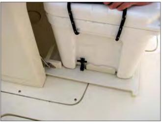
Cooler Slide Assembly & Draw Latch
