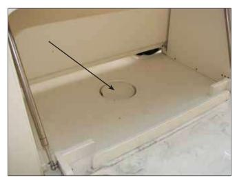
Fuel Tank Level Sending Unit Access Hatch
