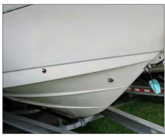
Bow Storage Compartment & Rope Locker Drains
