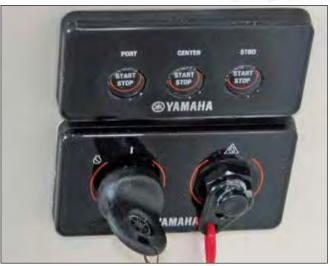
Typical Yamaha Triple Engine Ignition Switch and Start Buttons
