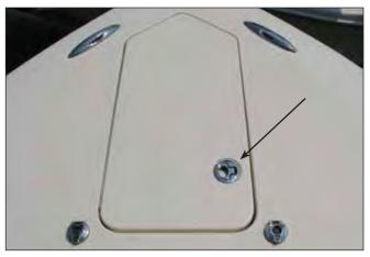
Anchor Locker Hatch Twist Lock Latch Handle can be stored flush to hatch only when latched
