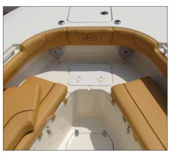
Anchor Rope Locker Hatch
