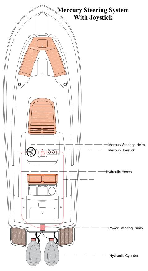
Mercury Steering System With Joystick
