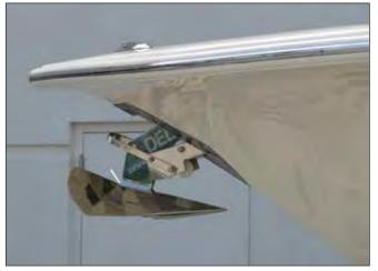
Anchor Roller & Delta Plow Anchor
