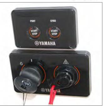
Typical Yamaha Key Switch, Start/Stop Buttons & Engine Stop Switch
