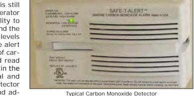
Typical Carbon Monoxide Detector
