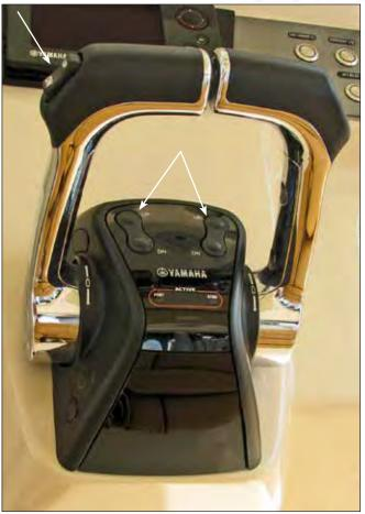
Typical Yamaha Engine Power Trim & Tilt Switches
