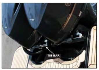
Typical Steering Cylinders & Tie Bar
