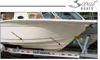
Forward Fishbox/Storage Compartment & Rope Locker Drains
