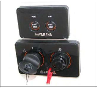
Typical Twin Engine Yamaha Command Link Plus Ignition & Start/Stop Switch System
