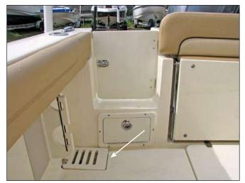
Starboard Cockpit Scupper Drain
