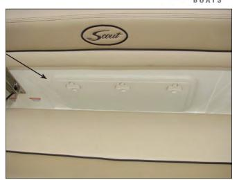
Aft Electrical Systems Compartment Hatch Behind Stern Bench Seat
