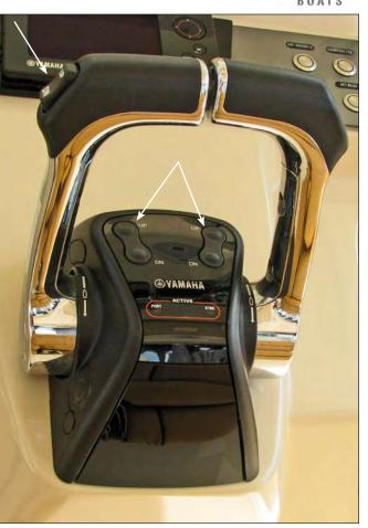
Typical Yamaha Twin Engine Trim & Tilt Switches
