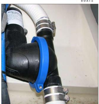
Typical Waste Discharge Diaphragm Pump
