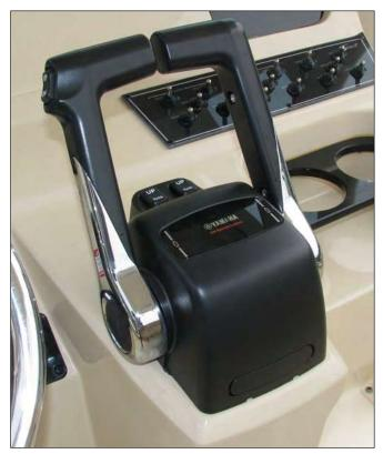
Typical Twin Engine Cable Controls
