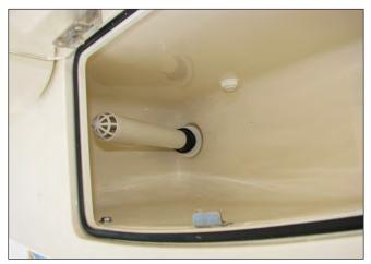
Leaning Post Baitwell Standpipe & Drain Fitting
