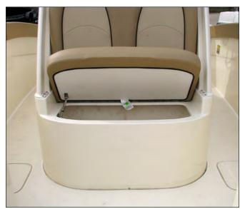
Forward Console Seat Cooler Hatch
