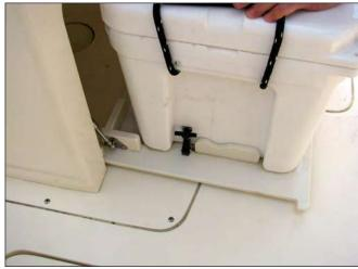
Cooler Slide Assembly & Draw Latch
