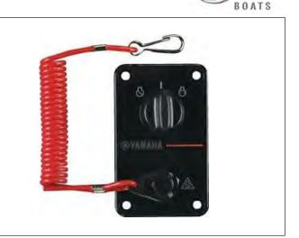
Typical Single Engine Yamaha Command Link Ignition Switch
