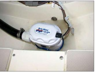
Bilge Pump W/ Built In Automatic Switch In Aft Systems Compartment
