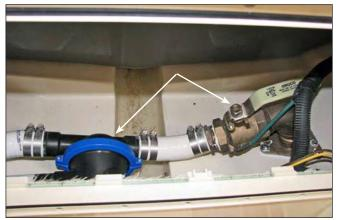
Waste Discharge Pump & Thru-Hull Valve
