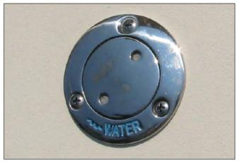
Fresh Water Deck Fill Plate Note: Press down and turn cap 1/4 turn counterclockwise to release and provide handhold
