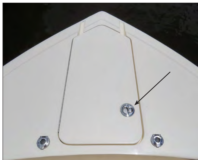
Anchor Locker Hatch Twist Lock Latch Handle can be stored flush to hatch only when latched
