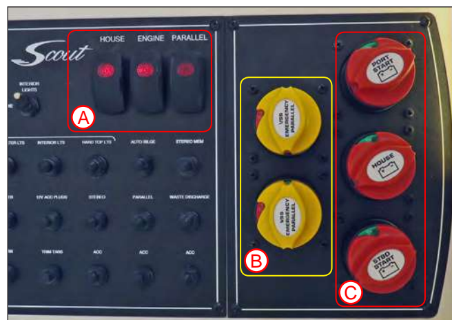
DC Panel Remote Switches & Main Battery & Parallel Switches
