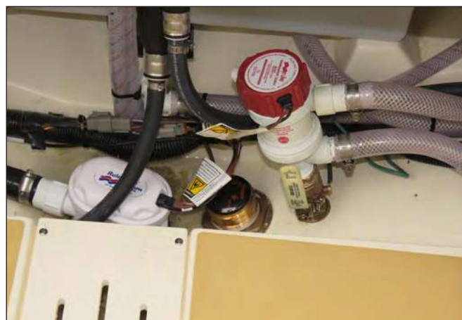
Baitwell Pump, Seacock Valve & Auxiliary Supply Fitting
