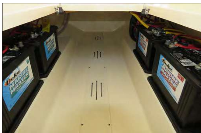
Typical Twin Engine Starting & House Batteries In Ski/ Battery Storage Compartment Below Cockpit Sole
