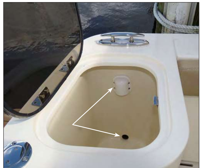
Baitwell Overflow & Drain Fittings
