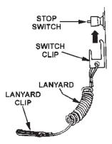
Figure B3: Emergency Engine Shut Off Switch
