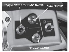
Figure D4: Digital Speed Control Switches
