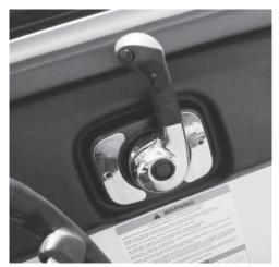
Figure D2: Throttle Control in Neutral Position
