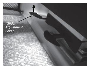
Figure C25: Bucket Seat "Slide" Lever
