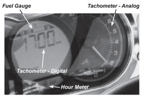
Figure B9: Fuel Gauge, Tachometers & Hour Meter
