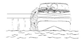
Figure A6: Minimize Exhaust Re-enty
