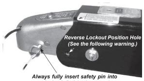
coupler latch (hole) prior to towing.
