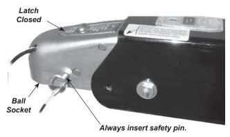
Figure F6: Brake Actuator & Coupling Assembly - Closed
