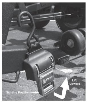
Figure F14: Rear Tie Down Strap - Tightening
