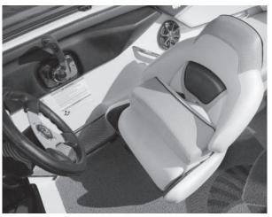
Figure C24: Bucket Seat with Flip-Up Bolster (Up)
