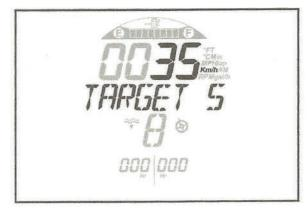
Figure D8: TARGET SPEED Displayed (Ski Mode)
