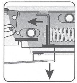
Figure F15: Emergency Break-Away System - Manual Release
