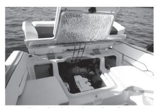
Figure C33: Raised Center Stern Seat -Engine Compartment Access
