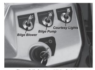
Figure B17: Starboard Helm Switches
