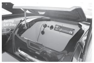
Figure C10: Port Console Glove box
