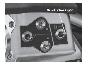
Figure B18: Navigation & Anchor Light Switch
