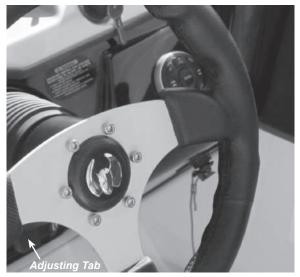
Figure B5: Tilt Steering Wheel (Adjusting Tab)
