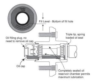
Figure F19: Turbo Lube Oil Fill Diagram
