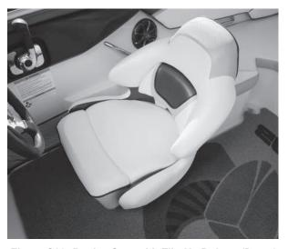
Figure C23: Bucket Seat with Flip-Up Bolster (Down)
