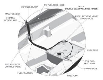
Figure B24: Pressurized Fuel System
