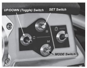
Figure B19: Digital Speed Control Switches
