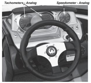
Figure B8: Information Center Gauges - Twin Engines
