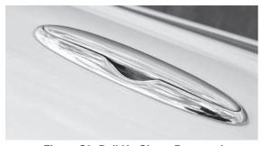
Figure C3: Pull-Up Cleat - Retracted
