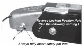
coupler latch (hole) prior to towing.
