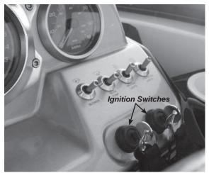
Figure B21: Ignition Switches - Twin Engine
