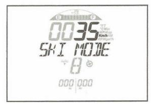
Figure D13: SKI MODE Displayed (w/Target Speed)
