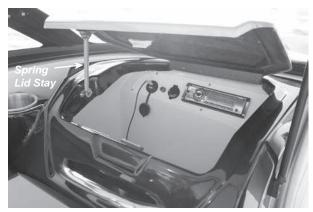
Figure C10: Port Console Glove Box
