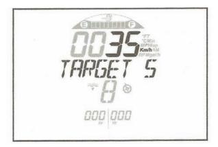
Figure D12: TARGET SPEED Displayed (Ski Mode)
