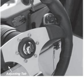
Figure B6: Tilt Steering Wheel (Adjusting Tab)
