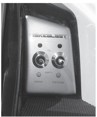
Figure B60: Ballast System Switch Panel
