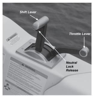
Figure D2: Separate Shift & Throttle Control
