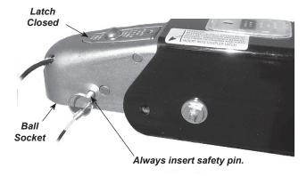
Figure F6: Brake Actuator & Coupling Assembly - Closed
