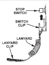
Figure B4: Emergency Engine Shut Off Switch
