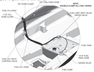
Figure B32: Pressurized Fuel System
