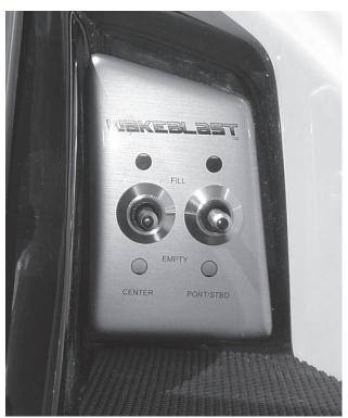
Figure B60: Ballast System Switch Panel
