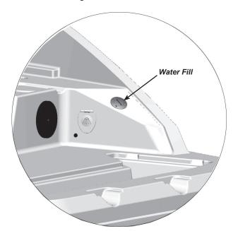
Figure B41: Water Fill - Starboard Transom
