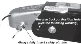
coupler latch (hole) prior to towing.
