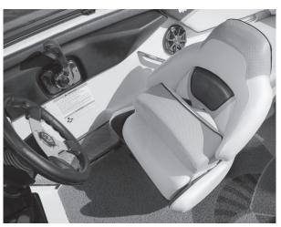
Figure C25: Bucket Seat with Flip-Up Bolster (Up)
