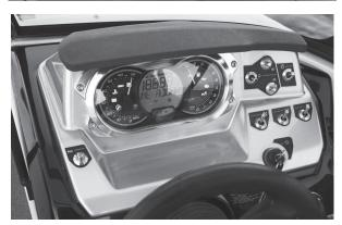
Figure B7: Information Center Gauges - Single Engine
