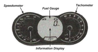
Figure B9: Information Center Gauge - Single Engine
