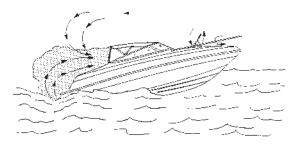
Figure B8: Backdrafting - Air flows over boat and behind transom
