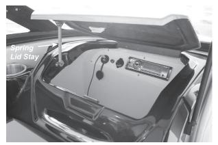
Figure C10: Port Console Glove Box
