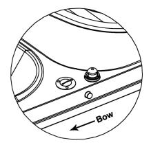
Figure B57: Pumpout Waste Deck Fitting
