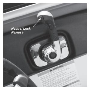
Figure D3: Throttle/Shift Control in Neutral/Idle Position
