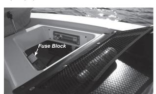
Figure B12: Fuse Block - Under Helm Console
