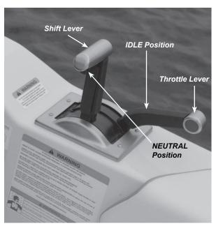
Figure D5: Separate Shift & Throttle Controls
