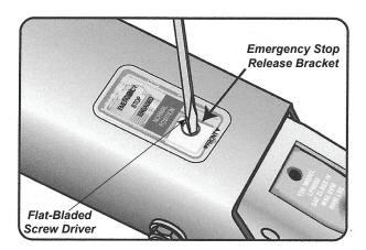
Figure F15: Emergency Break-Away System Manual Release
