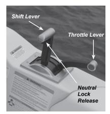
Figure B1: Throttle and Shift Lever Controls
