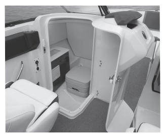
Figure B49: Enclosed Head (Applicable Models Only)
