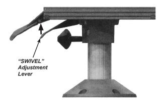
Figure C27B: "Swivel" Lever - Release to Rotate (Certain Models Only)
