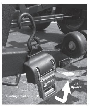
Figure F13: Rear Tie Down Strap - Tightening
