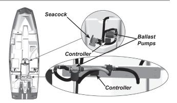
Figure B59: Pumps, Controllers & Seacock Location
