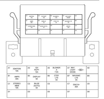
Figure B13: Fuse Block with Fuse Schedule (Applicable Models Only)
