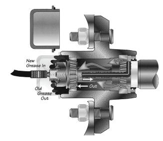
Figure F19: Vortex Lubrication System (Adding Grease)
