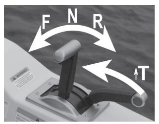
Figure D4: Separate Shift & Throttle Control Operation
