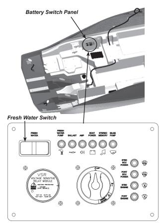
Figure B44: Fresh Water Switch on Battery Switch Panel
