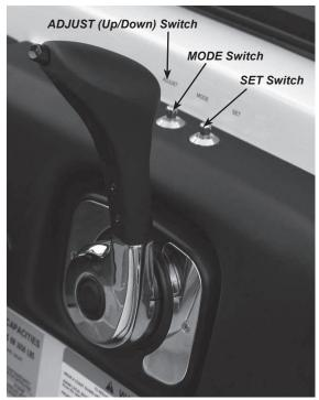
Figure D8: Digital Speed Control Switches - Armrest
