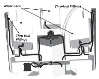
Figure B58: Ballast Water Sacs & Thru-Hull Fittings
