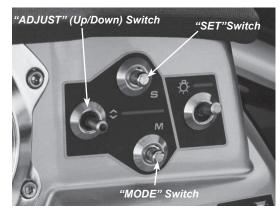
Figure D7: Digital Speed Control Switch
