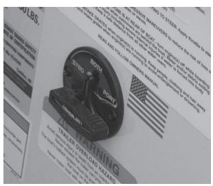
Figure B61: Port/Starboard Ballast Selector Switch
