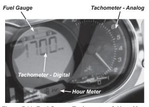
Figure B11: Fuel Gauge, Tachometers & Hour Meter
