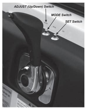
Figure B27: Digital Speed Control Switches - Armrest
