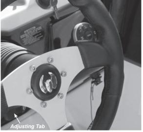
Figure B6: Tilt Steering Wheel (Adjusting Tab)
