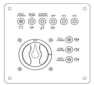
Figure B15: Battery Switch Panel - Single Engine (Battery Switch Panel May Vary Depending on Model)
