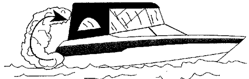
Figure 2.3 Exhaust Accumulation While Canvas is in Place
