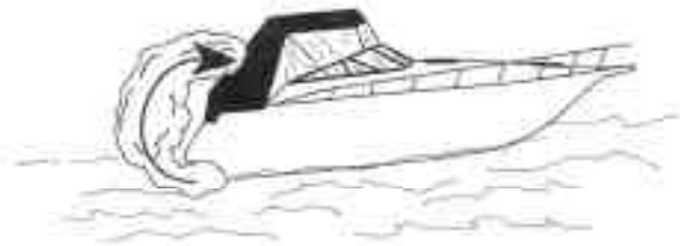
FIGURE 2.3 CO ACCUMULATION WITH PROTECTIVE COVERINGS
