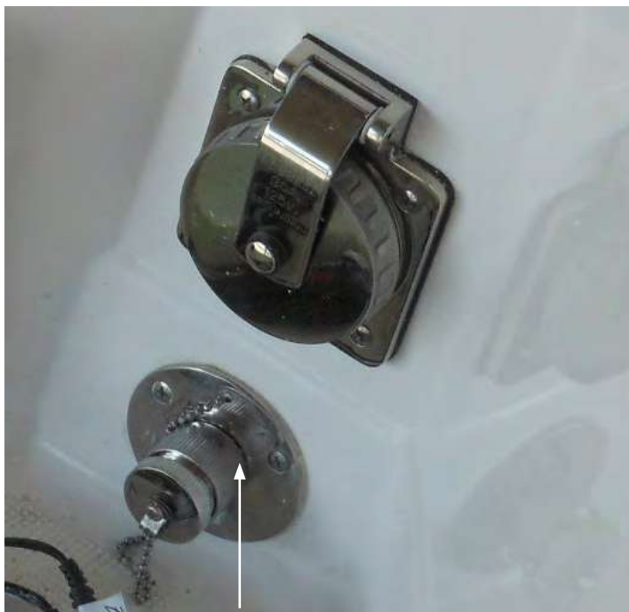
TYPICAL DOCKSIDE WATER INLET
