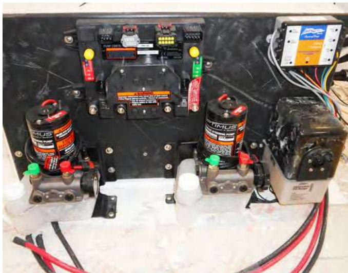
TYPICAL POWER STEERING BOARD
