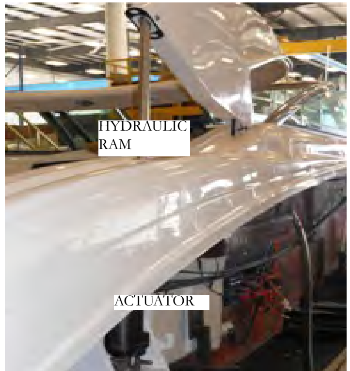
TYPICAL POWER TOWER IN FWD. POSITION
