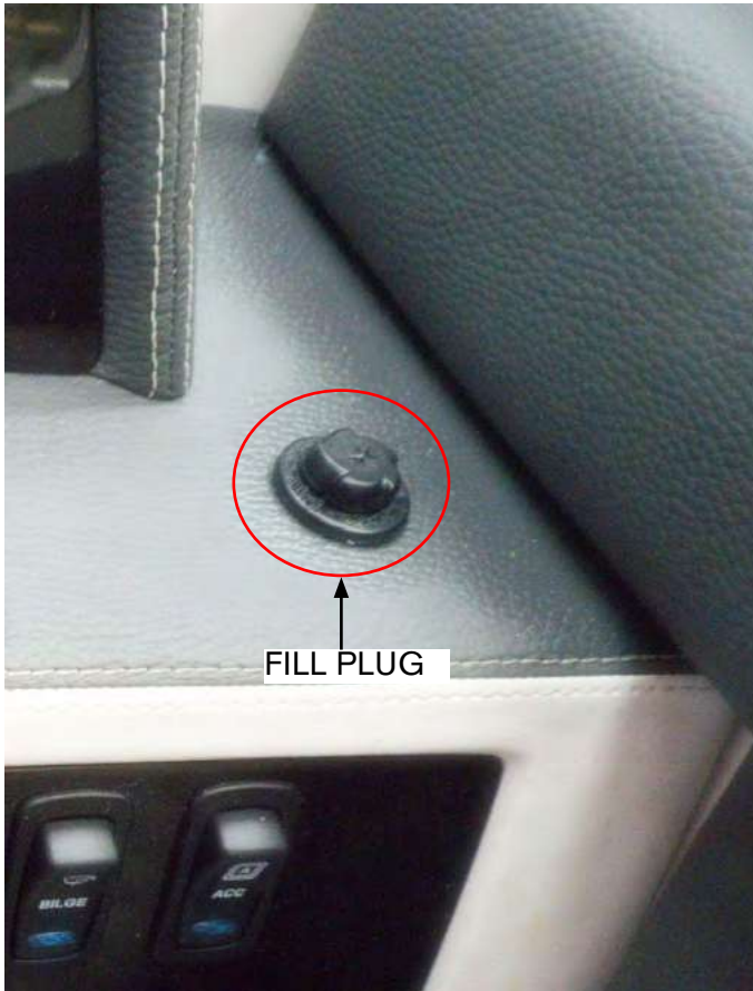
FILLING HELM HYDRAULIC STEERING FLUID
