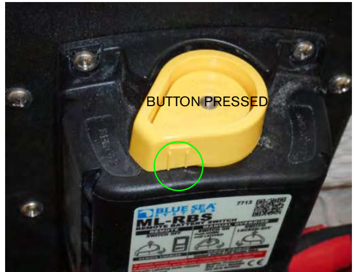
REMOTE BATTERY SWITCH- ON OR REMOTE POSITION-(NOTE ALIGNMENT MARKS)
