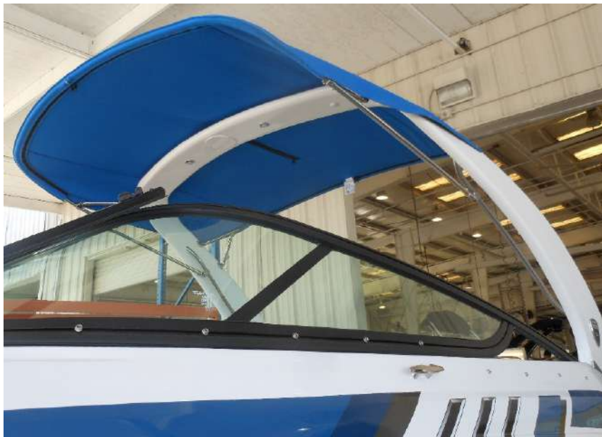
Typical Bimini Top/ Sunshade With Power Tower
