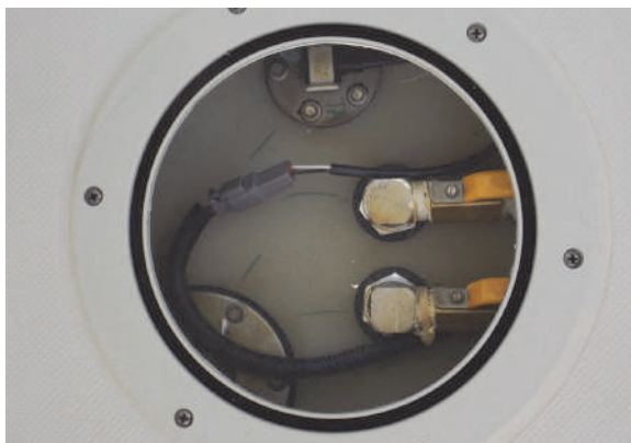
Gas Tank Valves
