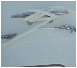
**Anchor Line Secured to Cleat**
