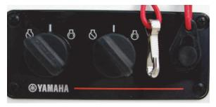
**Engine Stop Switch Lanyard (Typical)**
