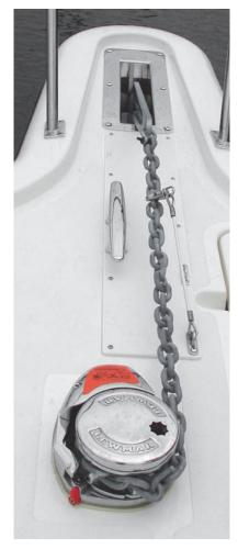
**Anchor Chain Properly Secured for Travel**
