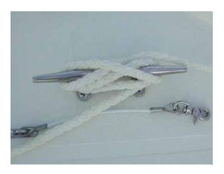
**Anchor Line Secured to Cleat**
