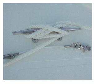
Anchor Line Secured to Cleat
