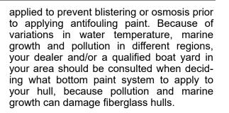
Sanding or sandblasting the hull bottom will damage the fiberglass. Only use standard antifouling paints and fiberglass wax removers and primers recommended by the antifouling paint manufacturer when preparing the hull for bottom paint. Sanding or sandblasting and the use of a coating other than standard antifouling paint or epoxy barrier coatings are not recommended and will void the hull blister warranty.
